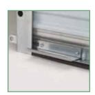
Tough, durable and wide, heavy duty nylon strapping helps control curtain stretch while deadening sound and reducing wear. The 11 gauge windlocks provide the strength to meet the stringent wind load requirements when engaged under load; however, easy operation is provided during load-free operation because the windlocks do not come in contact with guide.
