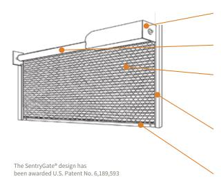
**BRACKETS** - Steel with powder coating in Gray. Bolt to guide assembly and support counter-balance shaft and curtain.
