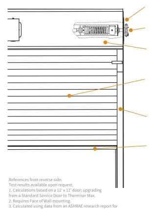
**BRACKETS** - Steel with powder coating to match the curtain. Bolt to guide assembly and support counter-balance shaft and curtain.
